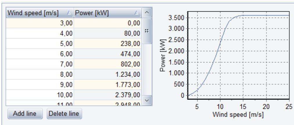
Figure 4. The power curve of the wind farm
