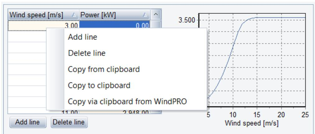
Figure 5. The power curve. Values can be copied via clipboard, including wind farm power curve calculated in WindPRO
