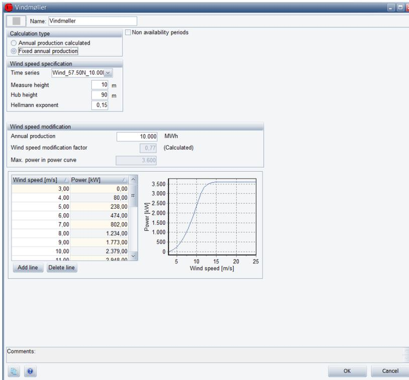
Figure 10. Fixed annual production (Scaling wind speed)
