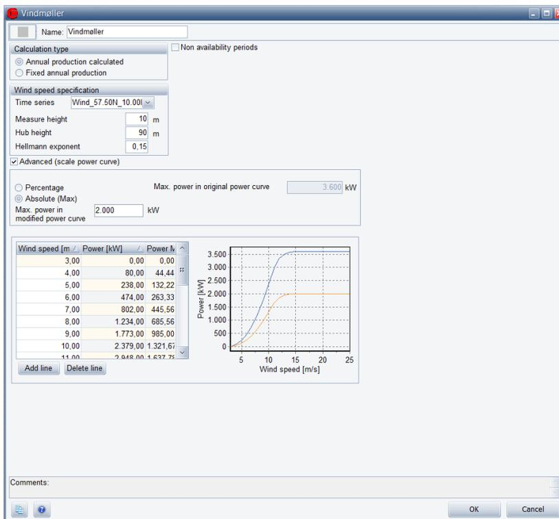
Figure 9. Wind farm, "Annual production calculated", power curve scaled with maximum power curve value
