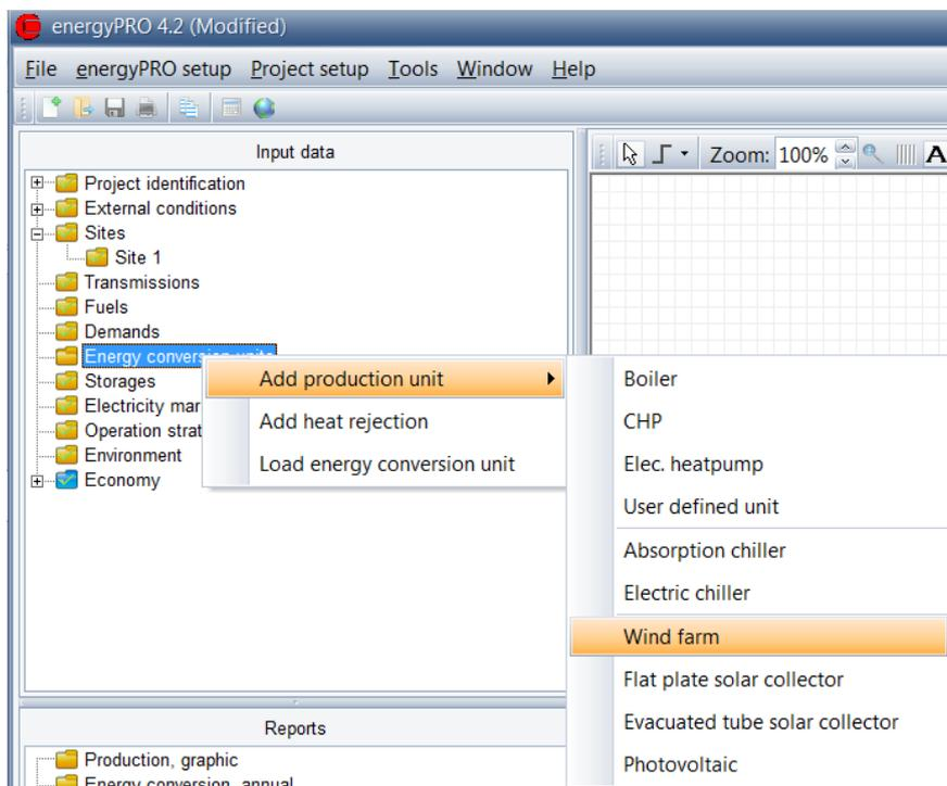
Figure 1. Select and specify the production unit - Wind farm
