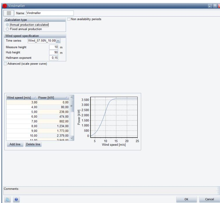
Figure 7. Wind farm, “Annual production calculated”, not advanced
