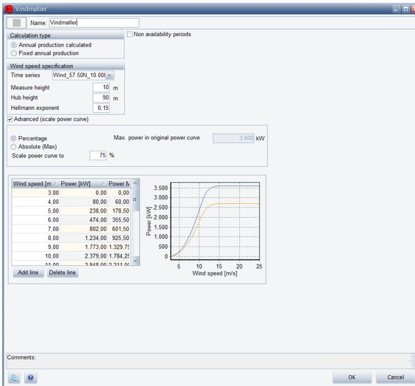
Figure 8. Wind farm, "Annual production calculated", power curve scaled with percentage
