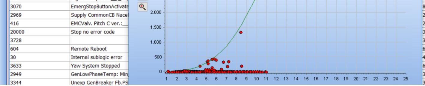
As example the above figure highlights events with an error code of 3273. This code represents all the events connected to cable CCW-untwist.
